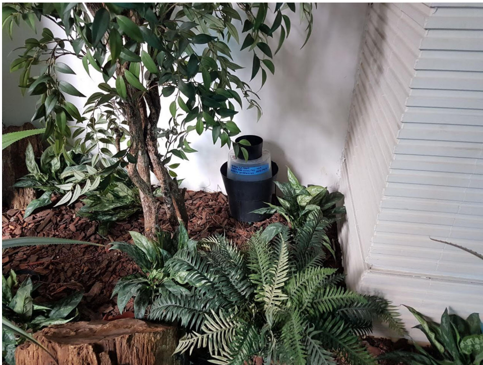
Figure 3. Photograph of gravid Aedes trap (GAT) setup in the field.
